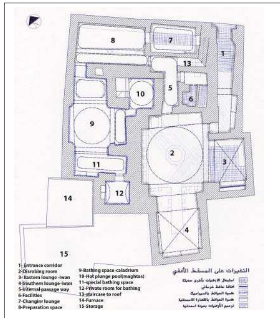
Figure 12: Plan of Samarah bath illustrating internal space. (Source: Autho rs).
